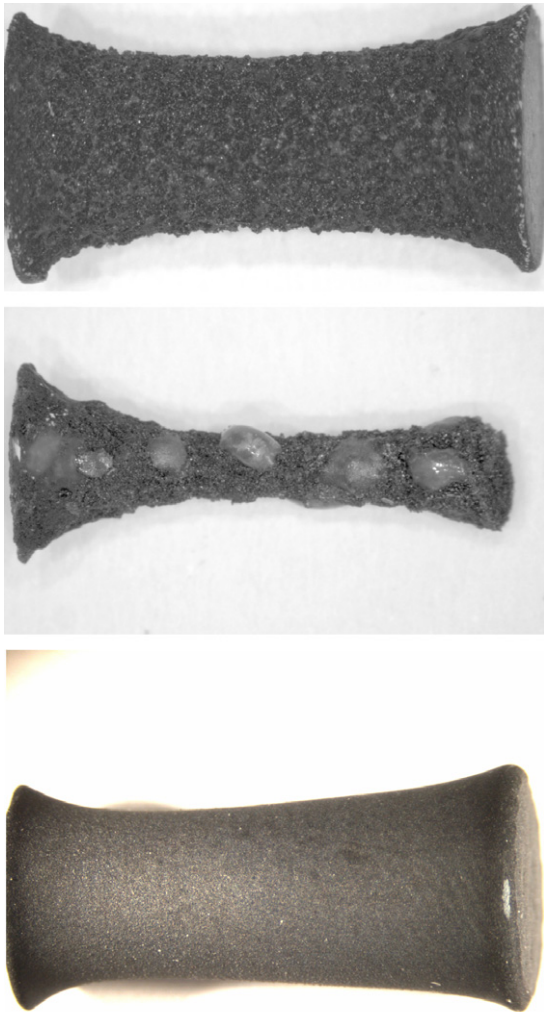
Fig. 3. Characteristic pellet's shape after oxidation: upper – moderately oxidised pellet at 1200 °C, centre – strongly oxidised pellet at 1400 °C, showing the formation of vitreous drops at pellet's surface and lower – pellet oxidised at 1800 °C.
